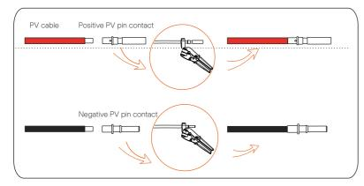
e. Insert the PV cable through fastening head and plug (male and female) and force the male or female plug to the cable. You will hear "Click" which indicates the connection is completed. Then tighten the fastening head.
