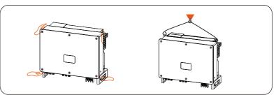
b. Hang the inverter on the bracket and secure it on the bracket with M8 bolts. (Torque: 7.0-8.5  $\rm N{\cdot}m)$
