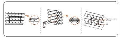
Step 2: Hang the inverter on the bracket
