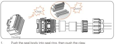
Push the seal body into seal ring, then push the claw.
