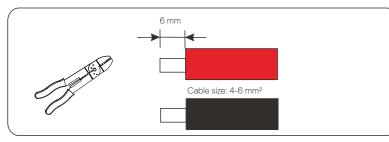
d. Tighten the stripped section and insert it into the PV pin contact. And use terminals press clamp to clamp it so that the stripped section of PV cable is in firm contact with PV pin contacts.
