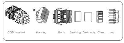
b. Select 0.5-0.75 mm2 conductor and use wire stripper to strip 12-14 mm insulation layer of the cable end and insert the insulated cord end terminal to the cable end. (ENY0512 nylon terminal for 0.5 mm<sup>2</sup>/22 AWG conductor; ENY7512 nylon terminal for 0.75 mm<sup>2</sup>/20 AWG conductor)
