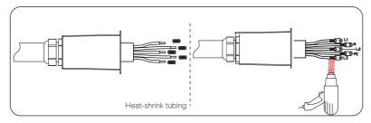
> Step 2: Connect the AC cable to the inverter
