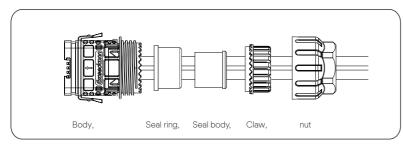
Insert the tube type terminal into the housing according to the label on e. it. Push the terminal-inserted housing into the body. There will be a slight sound of "Click", which indicates the connection is completed.
